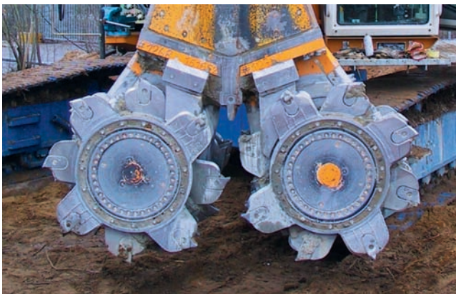
Type 3-1 (four tooth holders in one row of teeth)
